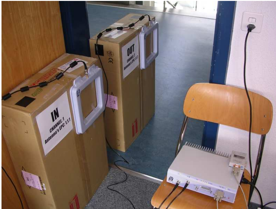
Figure 5.12.: A concrete example of capturing the direction of the motion
