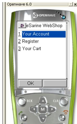
Figure 4.4: The same WALL markup as in 4.3 on Openwave 6, notice that the search form is not being displayed as these methods are not supported by WML 1.x, a work-around to this problem is proposed in chapter 8.
