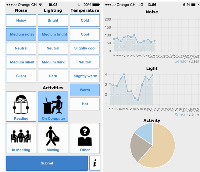
Figure 2: Smartphone application form to acquire perceived comfort (left) and the representation of the data recorded compared with objective data from sensors (right)
