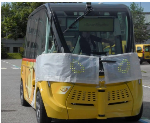
Fig. 3. The Intent Communication Interface attached to the driverless shuttle, and displaying the Anthropomorphic signal corresponding to intention Running NOW & will STAY Running (see Table 1).
