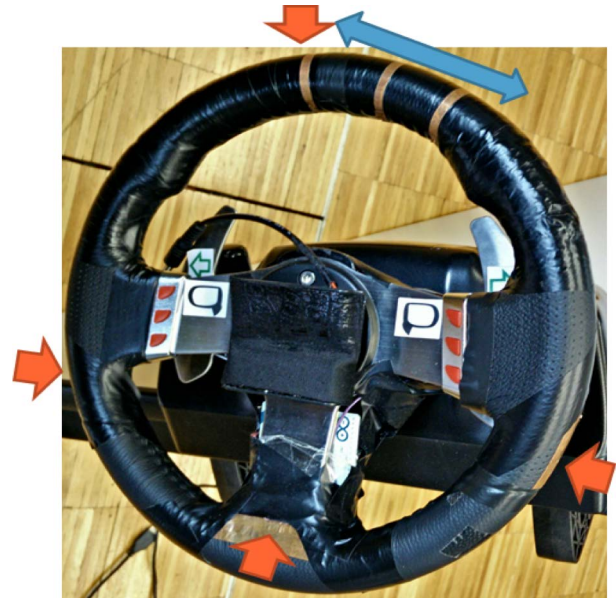
Figure 2. Logitech G27 Steering Wheel equipped with capacitive sensors, also called WheelSense. Red arrows depict hand-taps and blue arrow the hand-swipe.
