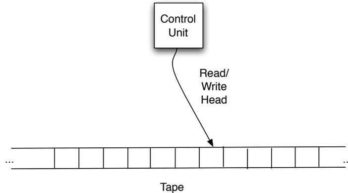
Figure 3.1: Turing’s machine: The control unit is at any time in determinate state. The read/write head is represented as an arrow which links the control unit to the tape
